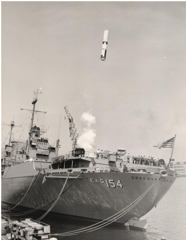
A dummy test Polaris missile is launched a short distance from a tube aboard USS Observation Island (EAG 154) at NNSY's Berth 42 in the late 1960s. The steam cannon-launched missile landed in the nearby Turning Basin. Credit Historic NNSY Archives
